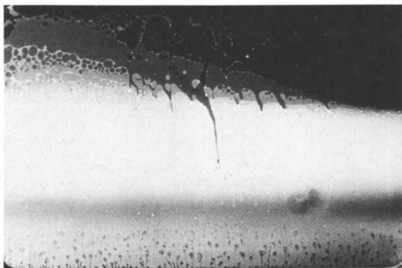
Plate 2. Stratified film of a NaDS solution in a different stage of drainage than the film of Plate 1
